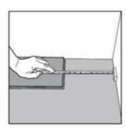
2.1. Start with a full plank and align the planks tongue with the working line, cut the last plank to the proper length leaving a ¼" from the end wall. Repeat this step for the second row, making sure to stagger the joints. The minimum end stagger is 6 inches.
