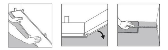
2.1. Start with a full plank and align the planks tongue with the working line, cut the last plank to the proper length leaving a <sup>1</sup>/<sub>4</sub>" from the end wall. Repeat this step for the second row, making sure to stagger the joints. The minimum end stagger is 6 inches.
